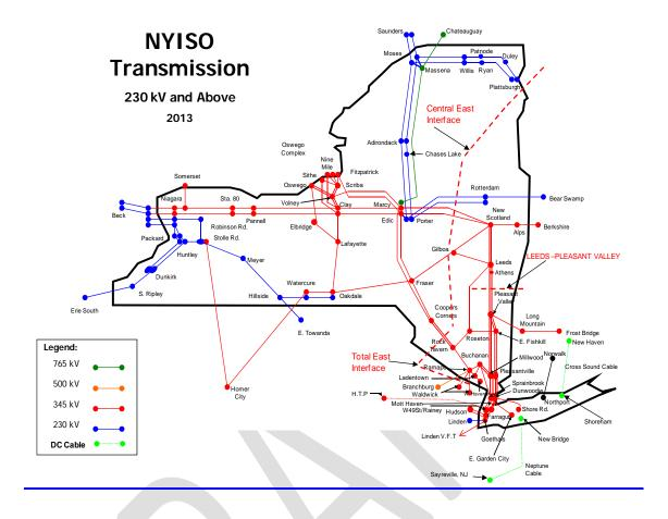
Figure 4-1: NYISO 230 kV and above Transmission Map
